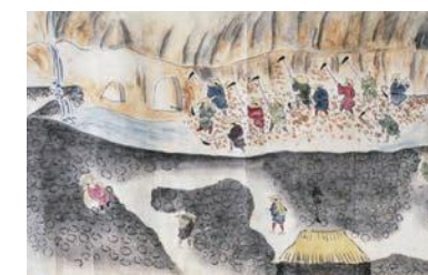
1) Scrape off the gravels containing placer gold toward the race built at the foot of the mountain.
