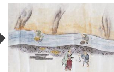
5) Put the collected sand on the Yuriita panning board and catch placer gold in the water with gravity concentration. It is tallied and sealed.
