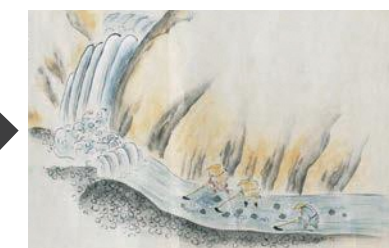
2) Dam up the stones in a row in the race and release the water from the reservoir to flush out the unwanted dirt. Heavy placer gold remains at the bottom of the race.
