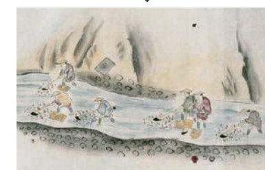
4) Gather the sand collected at the bottom of the race on Nekoda mat, a woven straw mat, and collect the minute sand by sifting through the mesh of the Nekoda mat.
